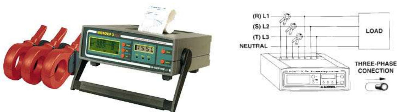
Figure 4.3: Three Phase Wattmeter and Typical Connection (Photograph: Elcontrol® Energy Net)
