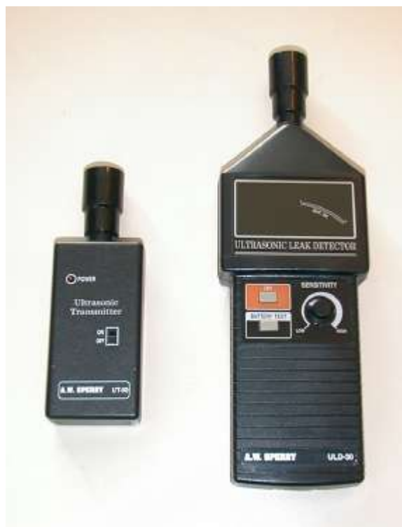
Figure 4.12: Ultrasonic Leak Detector and Transmitter
