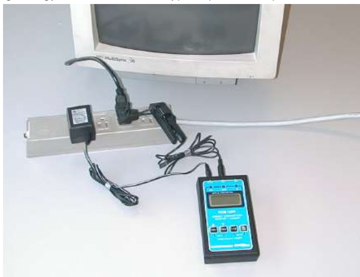
Figure 4.4: The Brultech ECM1200 Measuring Computer Monitor Energy Consumption
