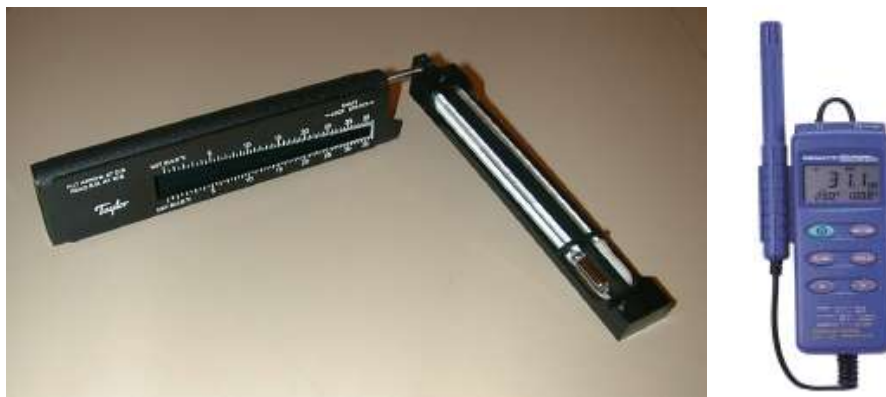
Figure 4.10 The Sling Psychrometer and Digital Humidity/Temperature Meter (Right Hand Photograph: ITM Instruments)
