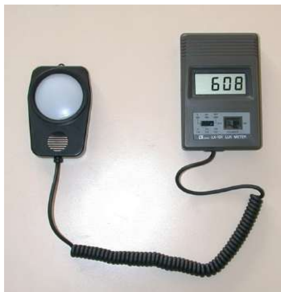
Figure 4.7: A Basic Light Meter
